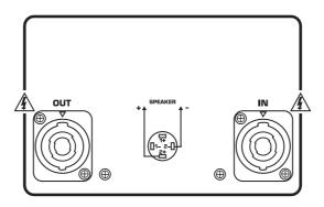
Fig. 1.2: Interface panel of subwoofer
